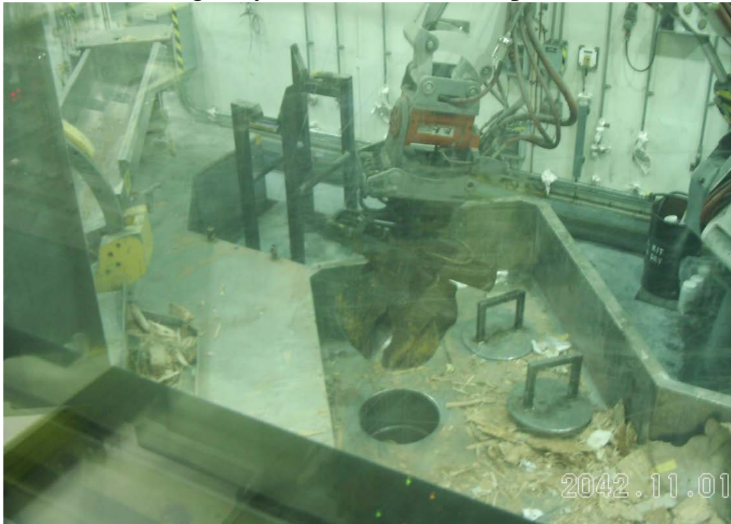
Boxline Sorting Tray with BROKK Manipulator
