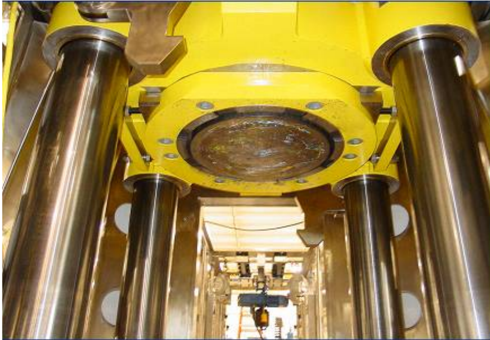
Supercompactor Ram
