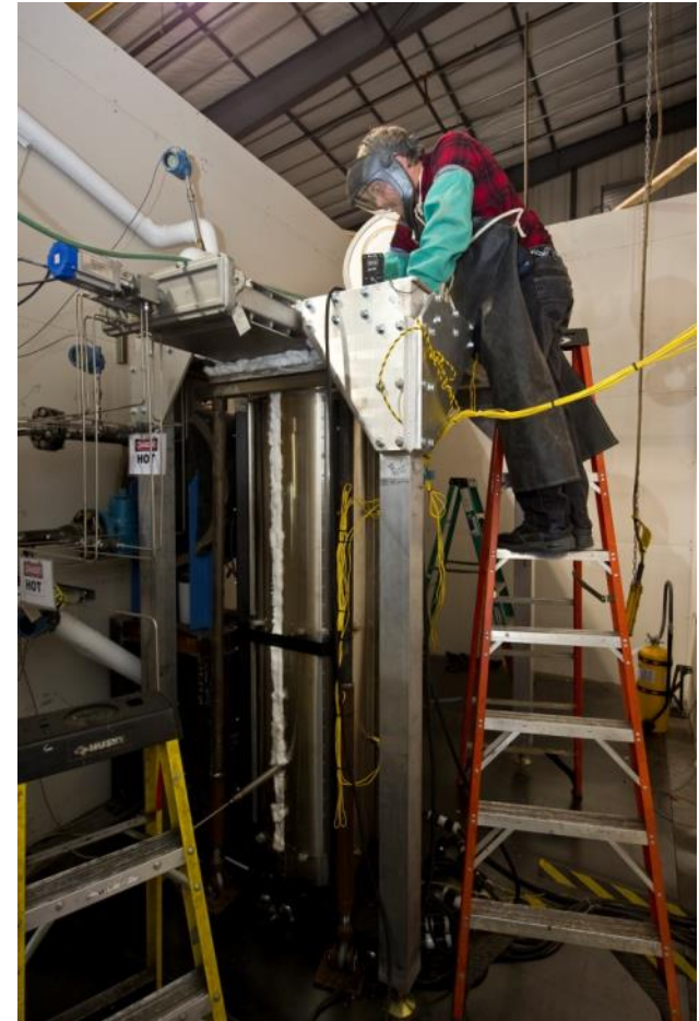
Sodium distillation equipment at Premier Technologies
