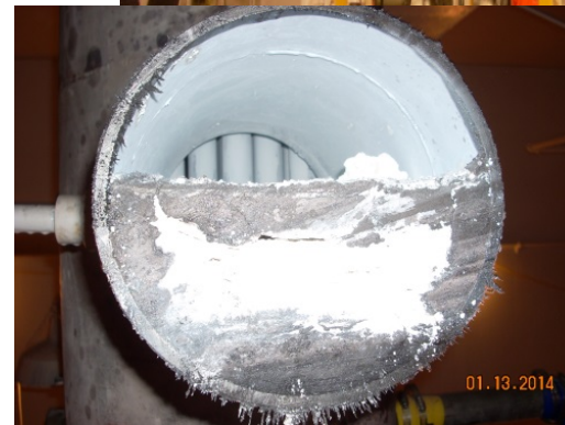
Removal of sodium-contaminated piping
