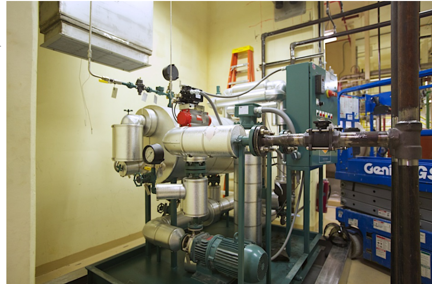
Assembly of sodium distillation equipment at INTEC
