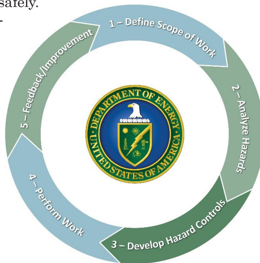
Figure 1. Integrated Safety Management is the system for safe work planning, performance, and continuous improvement at DOE.
