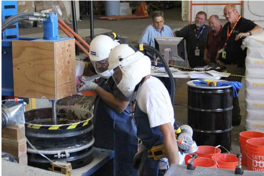
Picture 2. Discussions on safety issues are incorporated into simulated work at the Advanced Mixed Waste Treatment Plant, including when workers learn procedures in mockup situations, such as a practice session on solidifying used hydraulic oil, pictured here. Involving SMEs in these observations and discussions is critical to identifying hazards and controls.
