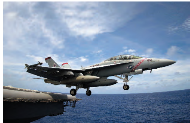
An F/A-18F Super Hornet launches from the flight deck of an aircraft carrier. (U.S. Navy photo by Photographer's Mate 3 rd Class Jonathan Chandler.)
