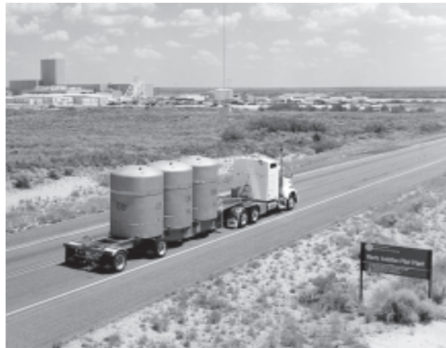
Truck carrying demonstration TRUPACT waste containers, with the WIPP site in the background.
