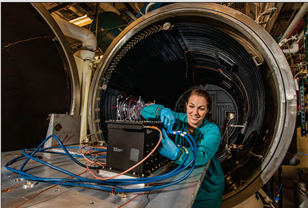
Researcher Rachel Trojahn prepares one of the boxes that makes up SNL's GBD for a test in the Labs' Flight Test Chamber. The chamber exposes individual boxes and the fully assembled flight system to the vacuum and thermal environment they will experience in orbit. (Photo: Randy Montoya)
