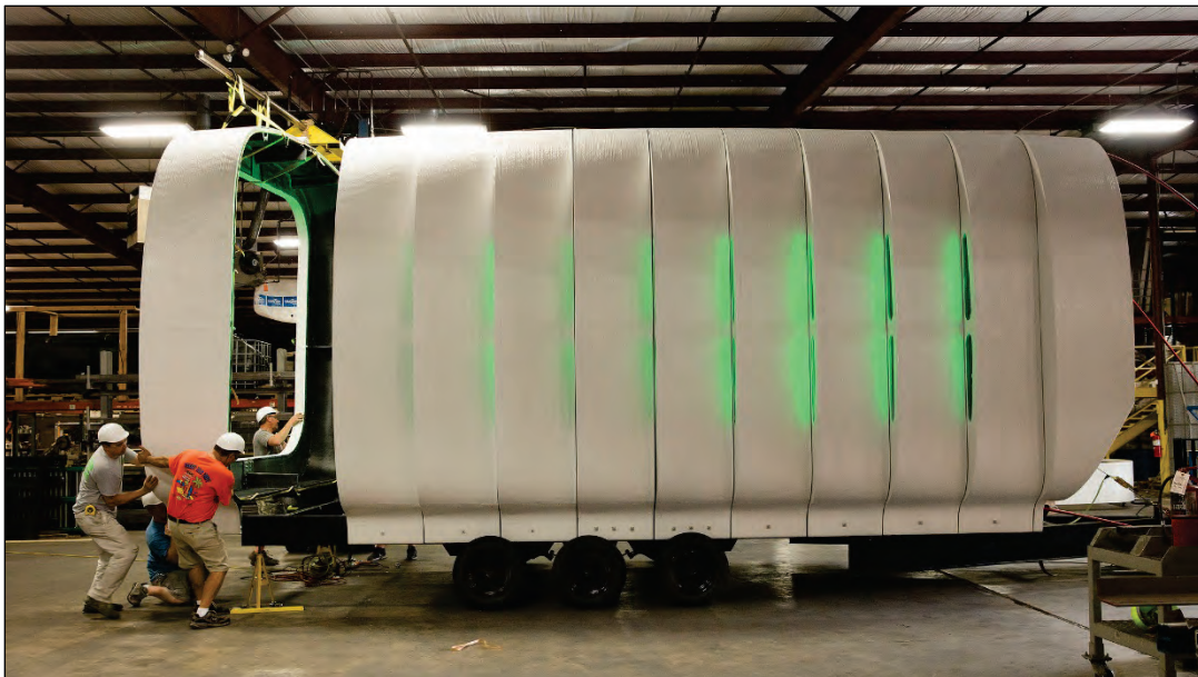
Figure 5. Structure Produced Using Additive Manufacturing (Oak Ridge National Laboratory, TN)
