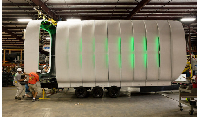
Figure 4. High-Performance Building Produced Using Additive Manufacturing at Oak Ridge National Lab
