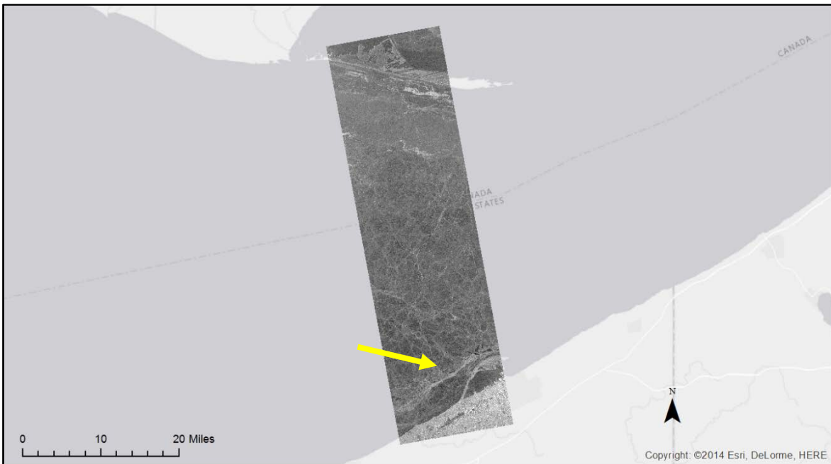
Figure 37. SAR image near Erie, PA, on 4 March 2015. The arrow indicates the position of a potential ice ridge. (Image ©DLR e.V. 2015, Distribution Airbus DS/Infoterra GmbH.)
