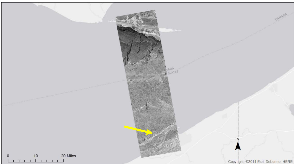
Figure 35. SAR image near Erie, PA, on 10 February 2015. The arrow indicates the position of a potential ice ridge. (Image ©DLR e.V. 2015, Distribution Airbus DS/Infoterra GmbH.)
