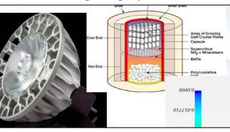
**Results to date**: HPC allows higher fidelity simulations showing more complicated flow structure, improved predictions of temperature and flow velocity in the reactor; now optimizing uniform growth of crystals
