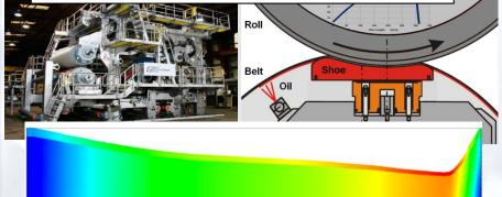
**Results to date**: Using both continuum and pore-scale approaches to determine how water flows through porous paper pulp; simulations can be used to optimize drying
