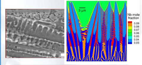
**Results to date**: Predicting crystal growth over large domains from multi-component alloys using phase field approaches; moving to new alloy systems and 3D
