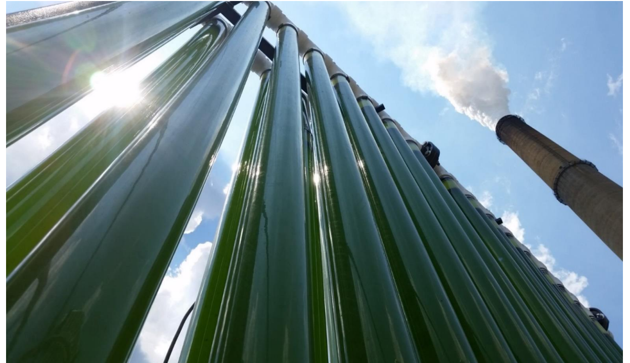
Pilot-scale “Cyclic Flow” Photobioreactor Duke Energy, East Bend Station, KY
