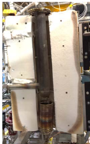
Bubbling fluidized bed reactor at NREL for biomass fast pyrolysis experiments.
