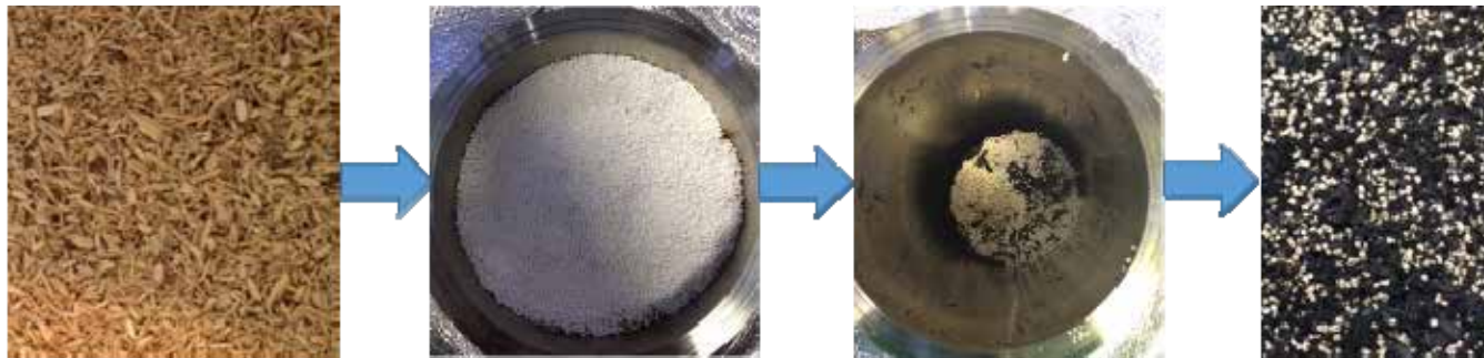
Photo from L to R: Fresh loblolly pine biomass, fresh biomass and co-loaded reactor, reactor post solvolysis extraction, remaining biomass and co-load
