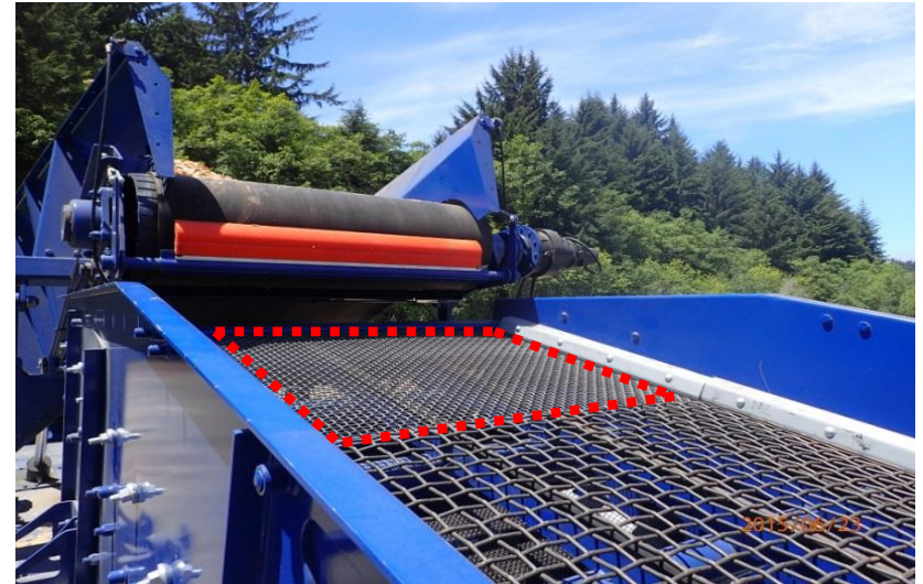
Screen Setting 2 (SS2); one 3/8 in. and 3 sets of 2 in. screens
