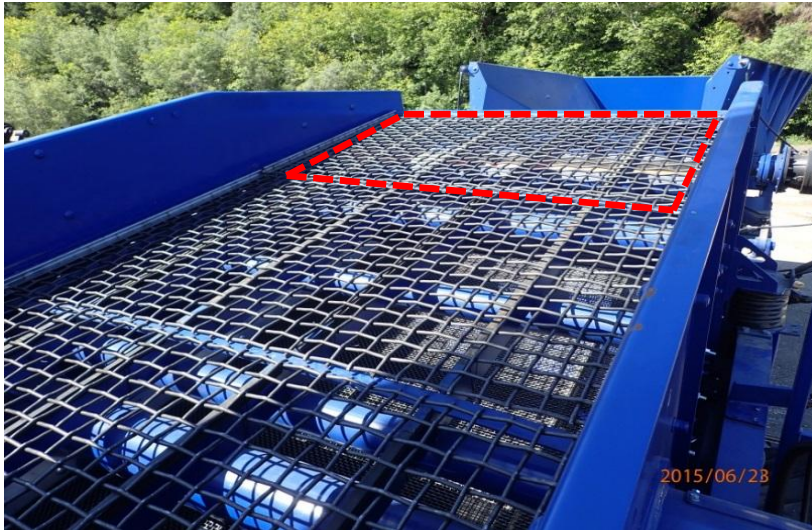
Screen Setting 1(SS1); 4 sets of 2 in. screens
