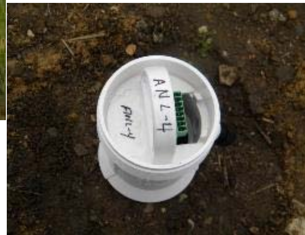
Profile soil moisture monitoring [10, 30, 60, 100, 120 cm depth]
