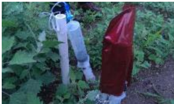
Soil-water sample collectors
