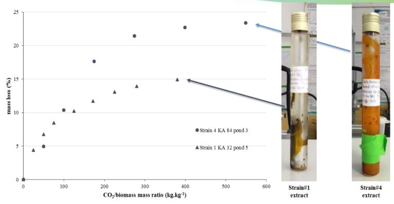
Comparison of extraction curves obtained from Nannochloropsis maritima (KA32) and Nannochloropsis salina (BR3) at 400 bar, 333 K and 0.5 kg\* $h^{-1}$ . >90% of neutral lipids and up to 80% of Omega-3 extracted using sCO<sub>2</sub>.
