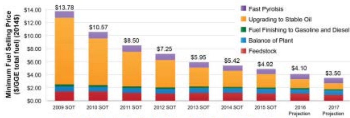
Figure 2-23: Cost projection breakdown for the fast pyrolysis design case
