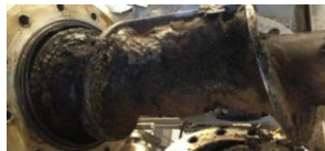
Accumulation of Coke and Chars
