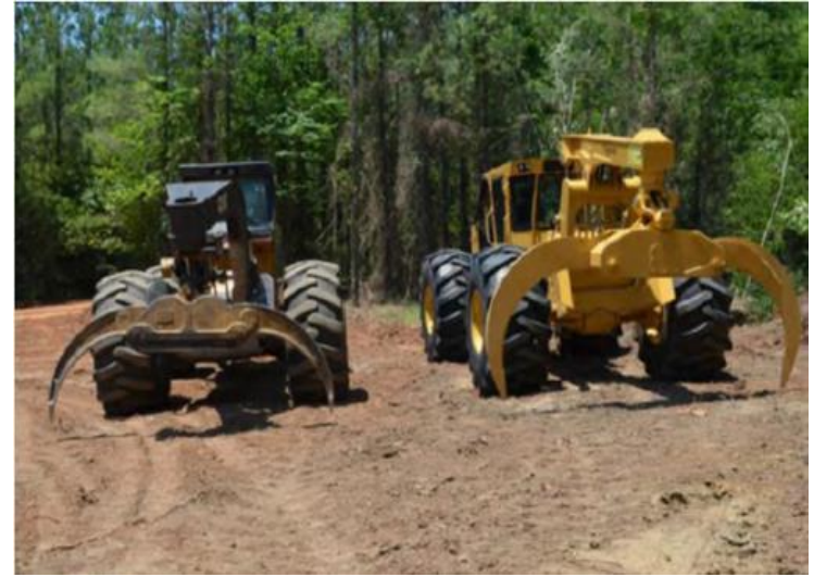
Enlarged grapple arms for the Tigercat wheeled skidder design developed through the DOE-funded Auburn University High-Tonnage Logistics Project
