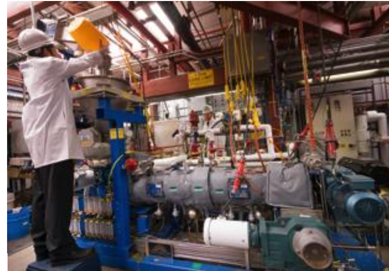
200kg/day, NREL horizontal pretreatment reactor
