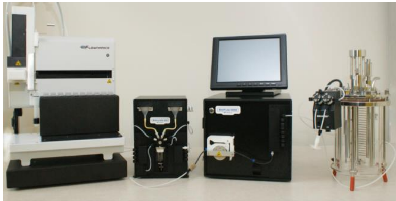
Flownamics 8000i system for high-frequency, 24-hour, cell-free sampling.
