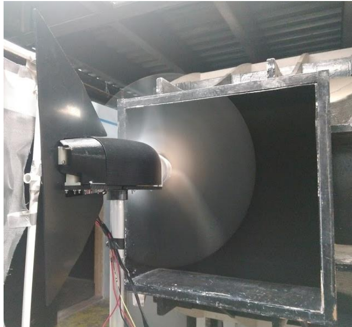
Figure 32: The spinning turbine looking down the mouth of the wind tunnel.
