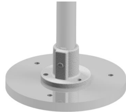
Figure 21: CAD drawing of the baseplate connection and tower.
