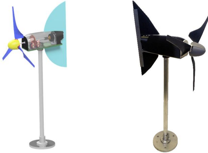
Figure 2: Competition turbine CAD rendering (left) and implementation (right).
