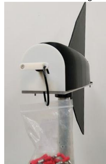
Figure 29: Turbine with installed lever arm and weights for torque measurements.
