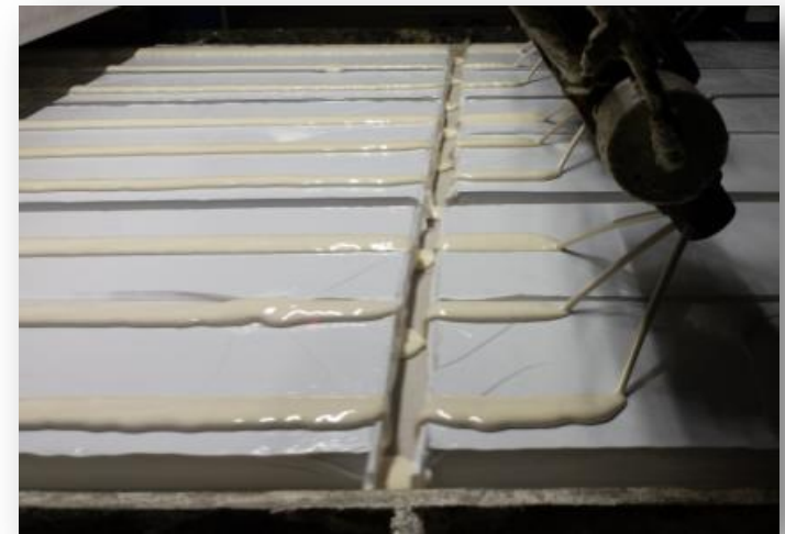
MAI-HD board fed through foaming line
