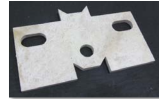
Long discontinuous glass fibers/PPS
