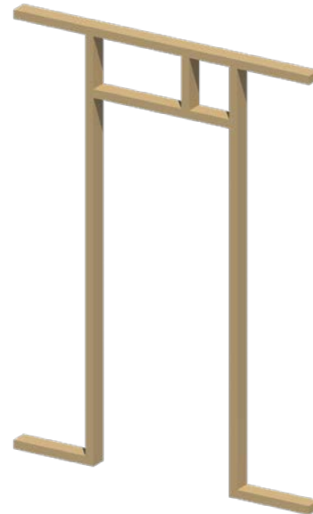
NON LOAD BEARING INTERIOR WALL
