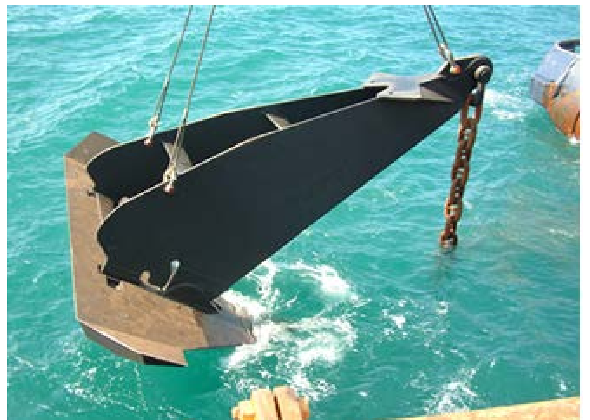
Example of a Drag Embedment Anchor.
