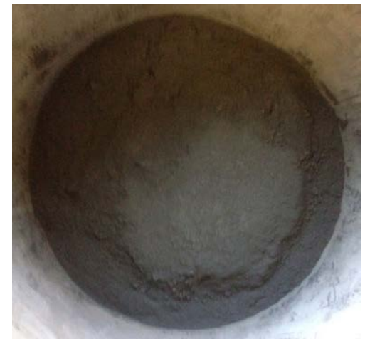
Taconite ore: 70% concentrate, <100 \mu\text{m}
