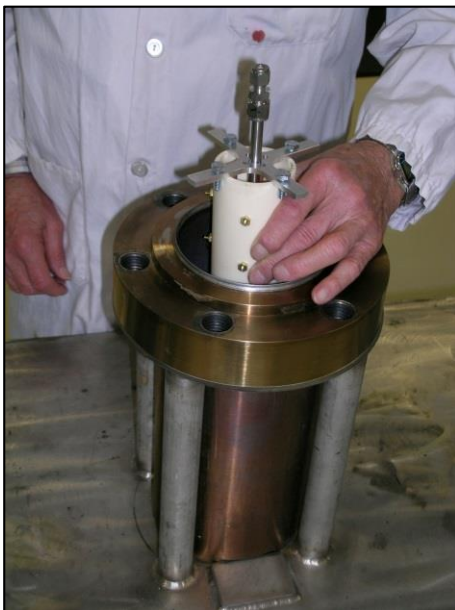
Boiling detector prototype testing in autoclave at HTTL
