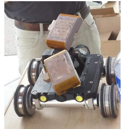
Magnetically coupled, side-looking ultrasonic sensor (Integrity Engineering, Inc.), on magnetic robot (Robotic Technologies of Tennessee)
