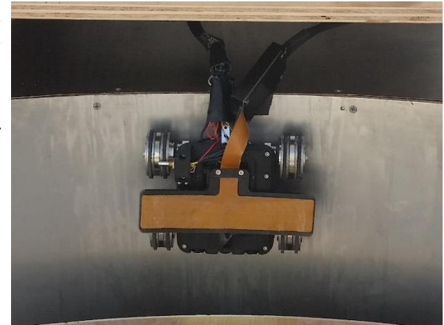
Flexible eddy current array sensor (Eddyfi, Inc.), on magnetic robot (Robotic Technologies of Tennessee)
