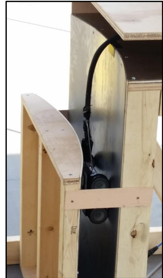
Robot rolls down overpack wall and enters annulus
