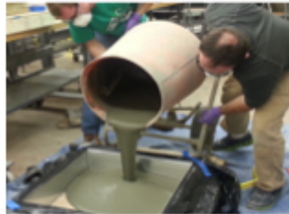
Pouring the cement into the mold
