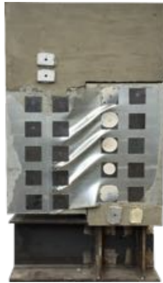
External Steel Plate \rho=0.25\% t=0.031 in. (22 gage)
