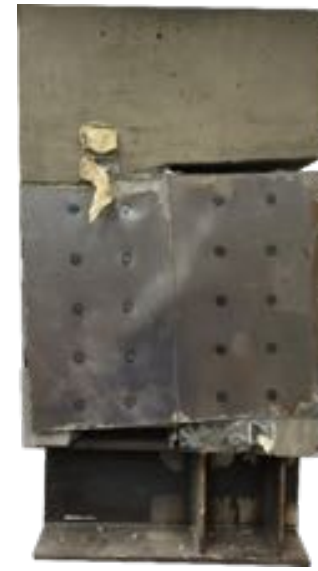
External Steel Plate \rho=0.75\% t=0.094 in. (13 gage)
