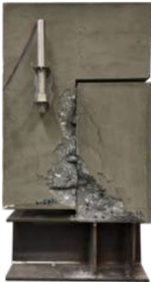
Internal Reinforcement \rho=0.75\%
