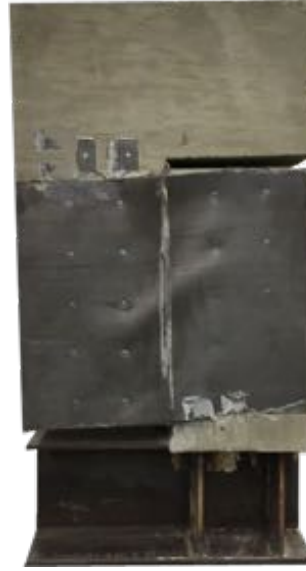
External Steel Plate \rho=0.50\% t=0.063 in. (16 gage)
