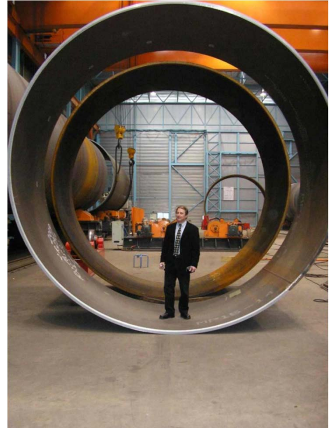
Carbon steel pipe welded with EBW Photo courtesy of TWI
