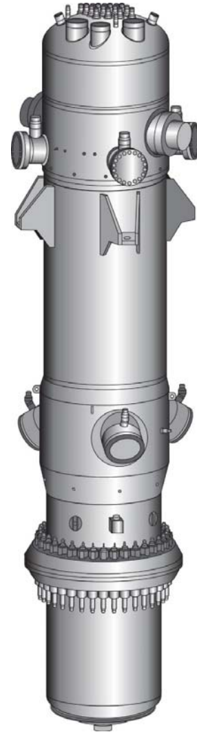
Representative Model of NuScale Power Reactor Vessel
