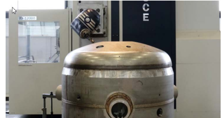
12m x 5m Horizontal Boring Mill Capability (Courtesy of N-AMRC)
