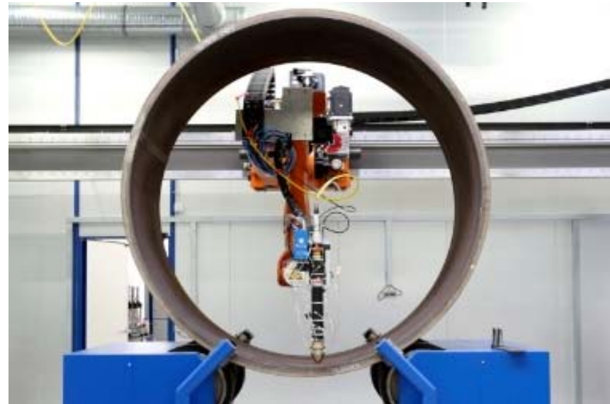
Diode Laser Cladding equipment setup (courtesy of N-ARMC)
