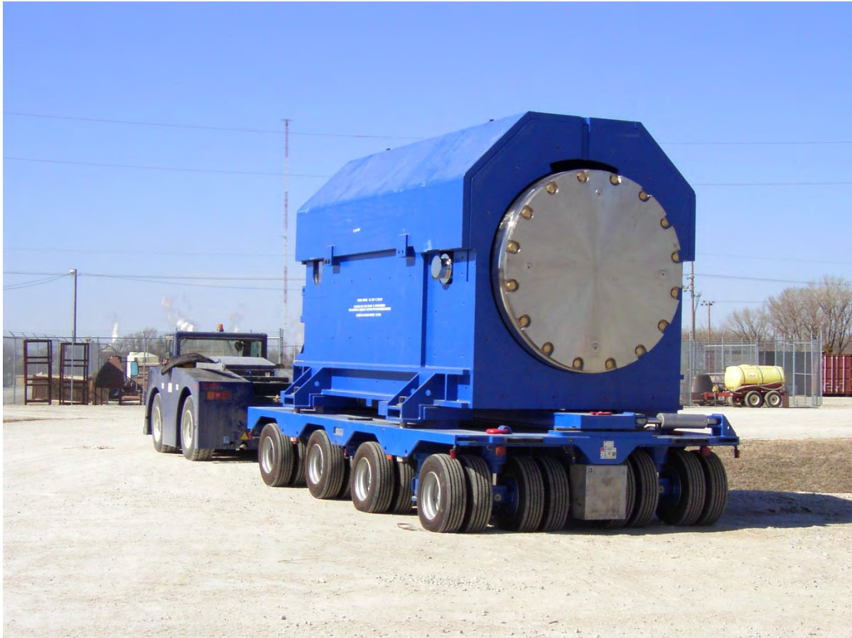
Figure 4-7 Removable Radiation Shielding on an AREVA TN Transfer Cask
