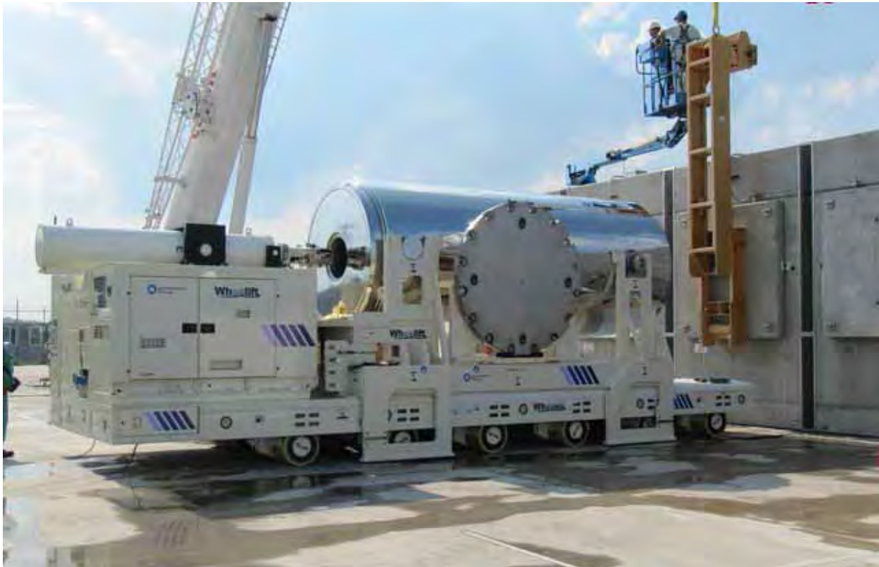
Figure 4-6 Wheelift Horizontal Cask Transporter for AREVA TN Systems
