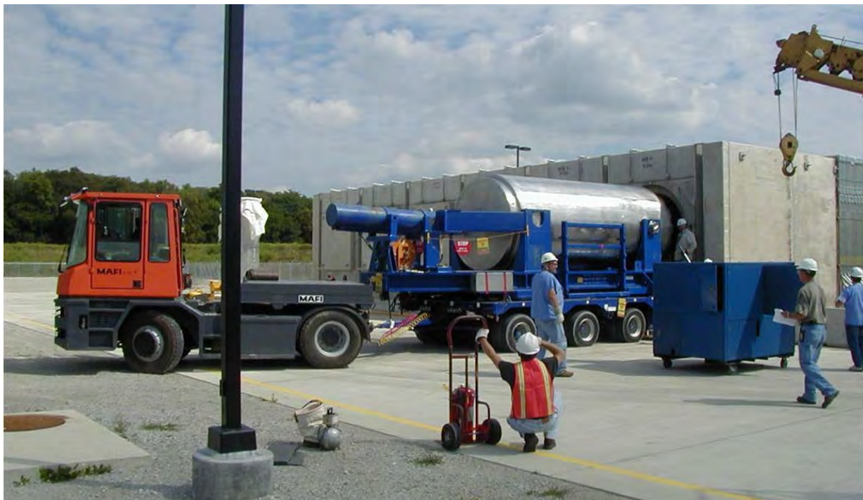
Figure 4-3 AREVA TN NUHOMS Horizontal Canister Transfer Using a TN Transport Trailer
