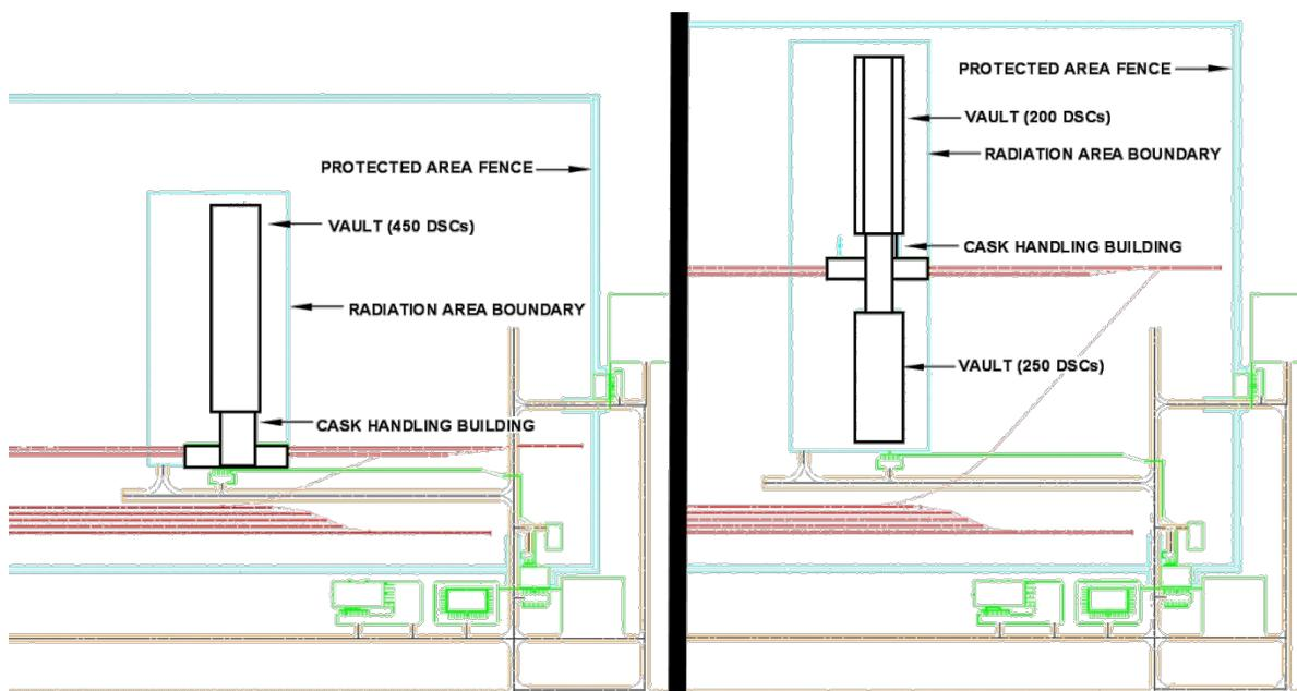
**Figure A4-4** shows the ISF site layout for below grade vaults with standalone CHB. As can be seen, the only difference in the layout of the site is the position of the CHB relative to the storage vault. It is also clear that because of the layout, the capital CHB can have two rail bays and independent OTB cranes.
