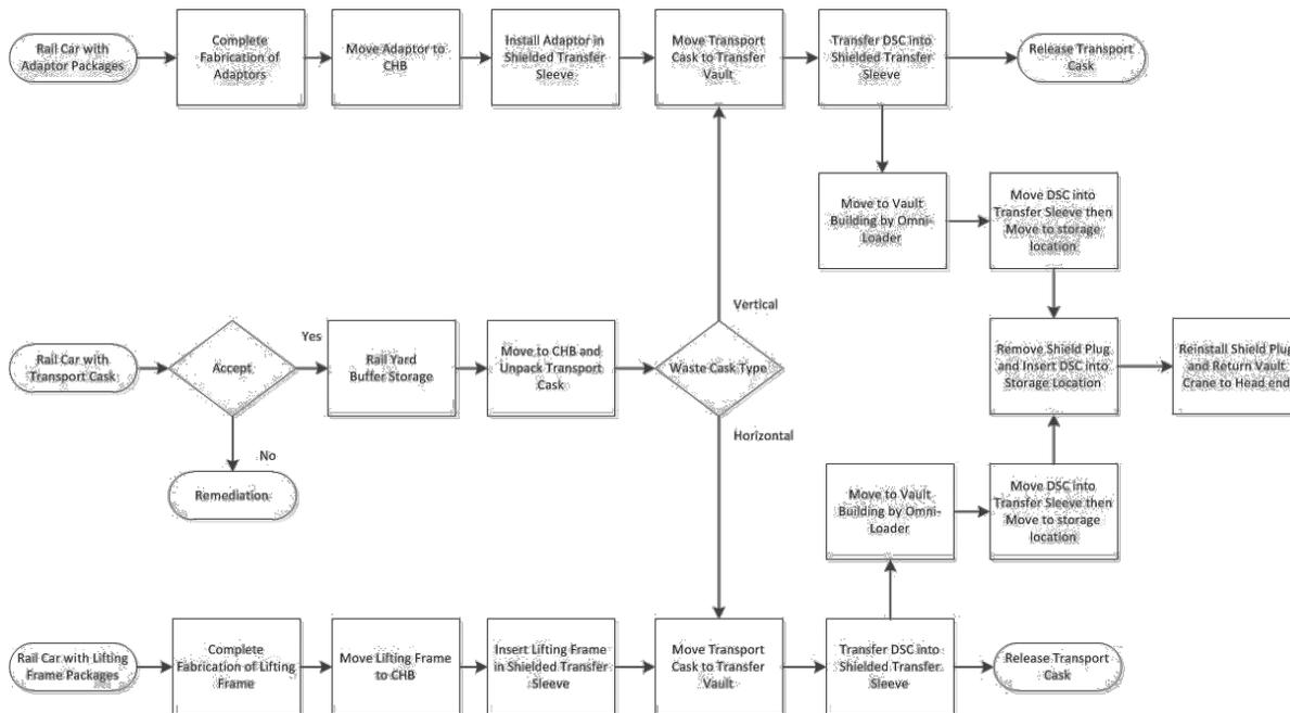
It should be noted that there are no significant differences in the processing times necessary for all-vertical versus vertical/horizontal storage designs. Minor differences in material needed and steps taken aside, the main differences among these designs is the ability to separate the processing of the Transport Casks from the storage of the DPCs. In other words, the options with an integral CHB vs the standalone CHB represent the only significant differences among these options.
