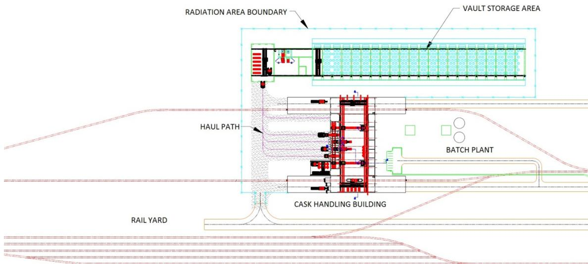
**Figure A4-5** shows the two configurations of the vault area with standalone CHB. BGVc is on the top; BGVd is on the bottom. It can be seen from these layouts that the expansion of the site is simplified by this approach and a wide variation of vault configurations could be added giving these variants broad capabilities for expansion.
