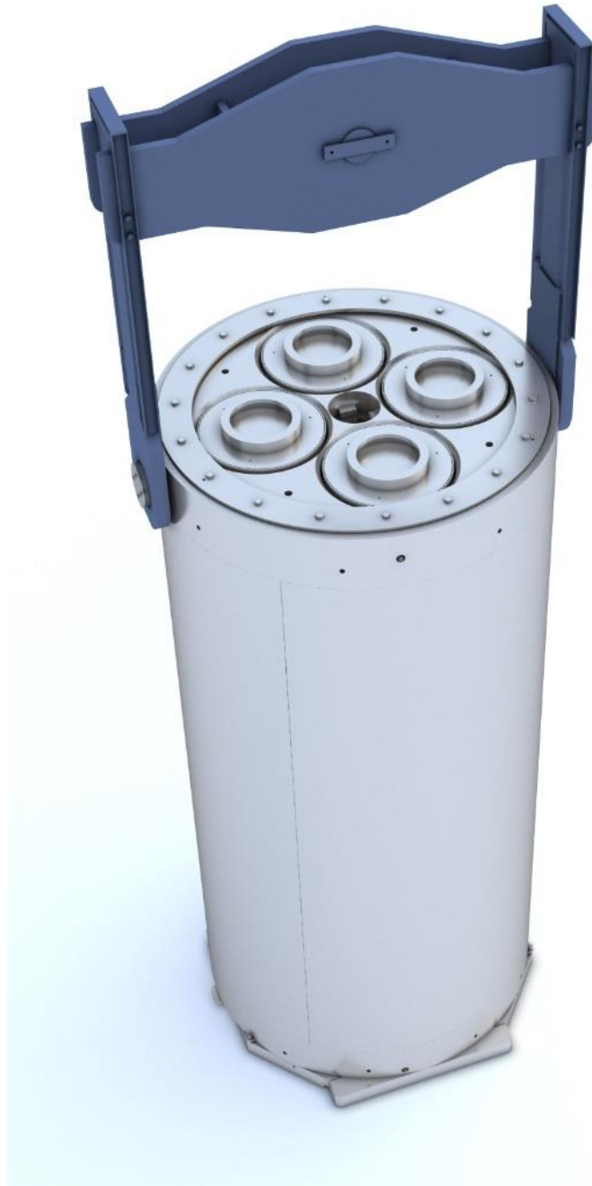
Figure 4-6. Loaded Carrier in Transfer Cask with Lifting Equipment
