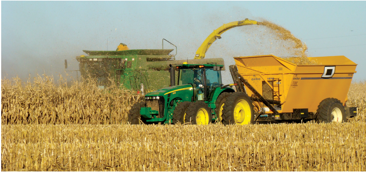
Figure 5 | A commercial-scale evaluation of the single-pass corn grain and stover harvest strategy in Minnesota (Image courtesy of Stuart Birrell, Iowa State University). Corn stover can be sustainably harvested provided corn grain yields are above 175 bu acre -1 . Note that the harvesting concept was developed from another funding source.
