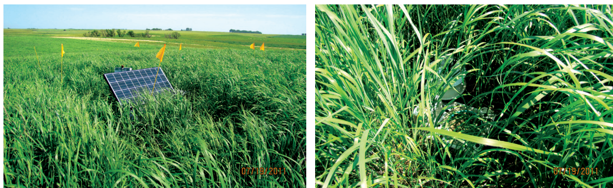
Figure 6 | Analyzer control unit with solar panel power ( left ) and static chamber ( right ) of an automated soil CO 2 flux system in a switchgrass stand during July (Image courtesy of Chang Oh Hong, South Dakota State University)
