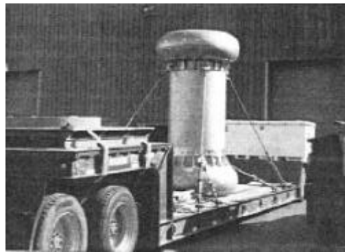
Type B cask used for transporting spent reactor fuel
