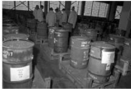
Type A packages are made of fiberboard, wood, or steel and often have some shielding material for LSA radioactive materials
