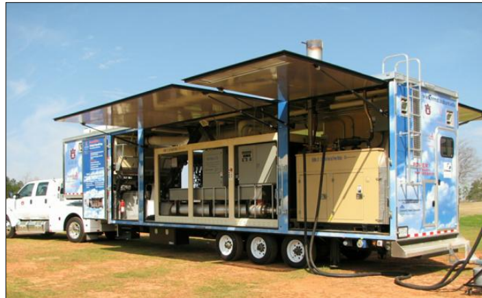
Pilot-scale (0.5 ton/day) Mobile Downdraft CHP
