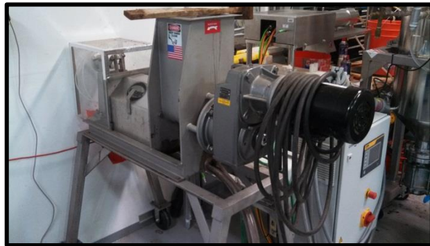
Screw Press Liquid/Solid Separation (NEW)
