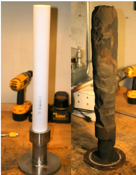
Fresh and Used (~1740 cycles) Ceramic filter element
