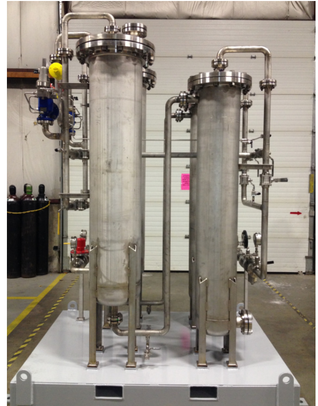
Lead-lag configuration with 6' x 6' skid for a 300 kW e system ~300L sorbent – 4 month operation
