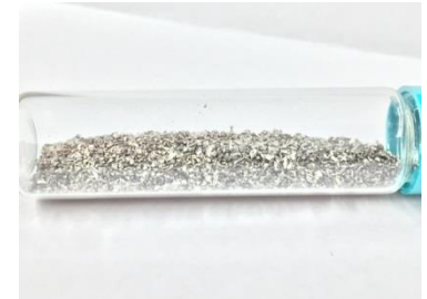
MCM particles are difficult to be manufactured to shapes and parts. They are fragile, heat sensitive, and very reactive
