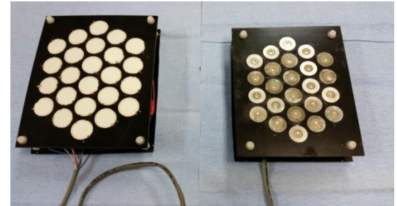
Drying 14 in 2 of fabric on matrix of 24 mesh transducers
