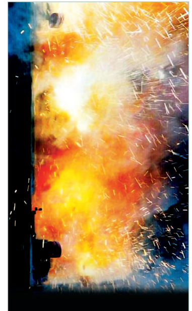
Figure 1-2. Energy released after a typical arc-flash event
