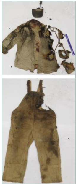
Figure 1-3. Clothing recovered after the arc flash event
