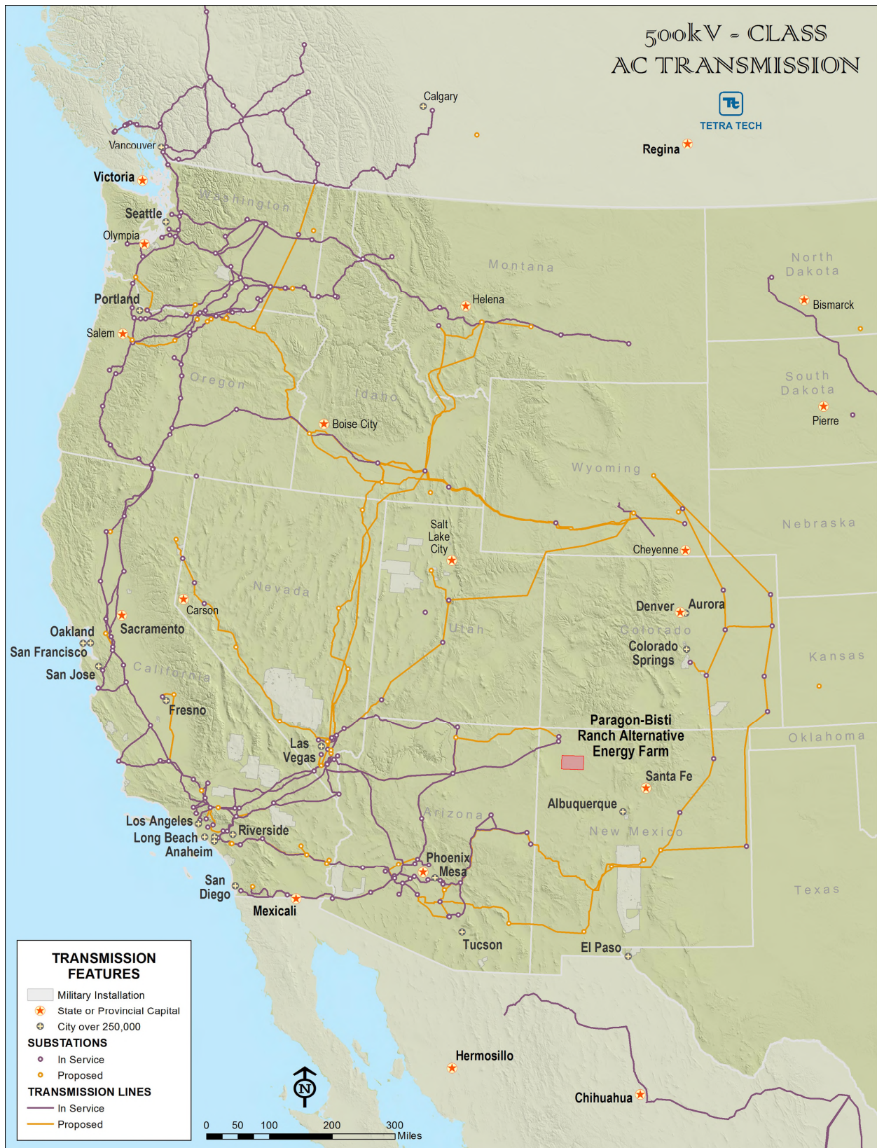
Figure 3-12. 500 kV-Class Transmission Infrastructure of the Western U.S.
