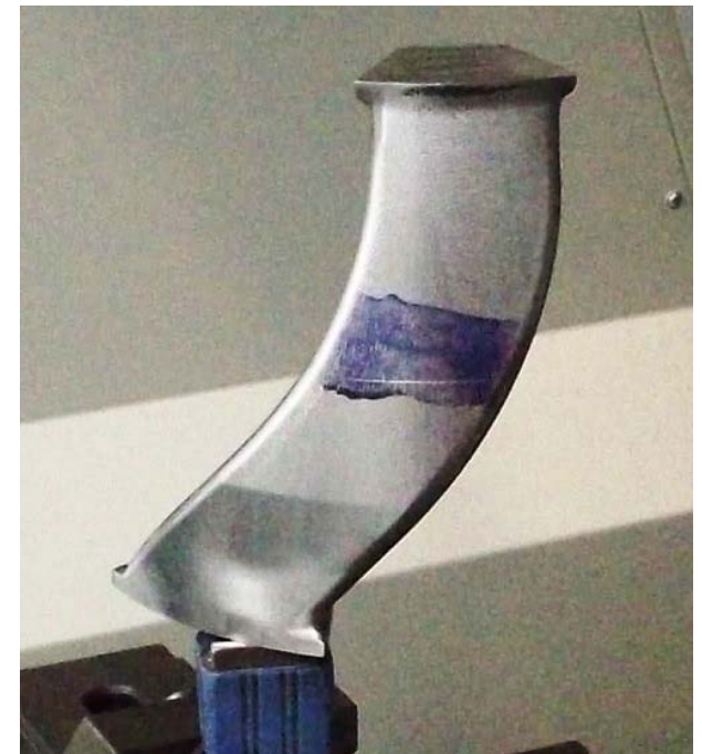
Vane Insert—one of 8 that fit into the swirler
