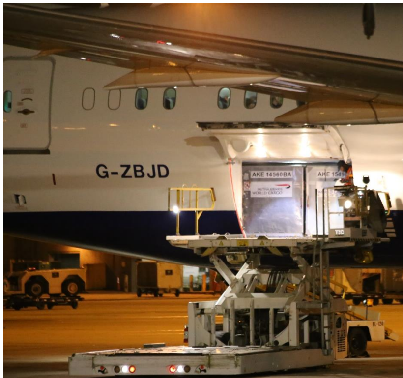
Figure 8. Airplane interior lighting compared to PHL HPS apron lighting. The cargo hatch of the airplane is raised, revealing the white color of the interior lighting as well as the supplemental lighting on the cargo loader. The yellow color of the PHL HPS apron lighting system can be seen below and on top of the plane.
