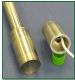
HT-TD before and after sealed for in-sodium test
