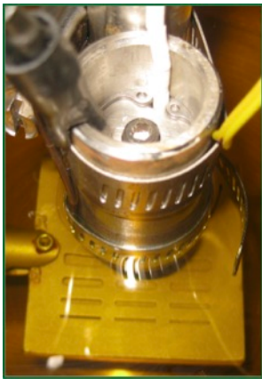
HT-TD before and after sealed for in-sodium test
