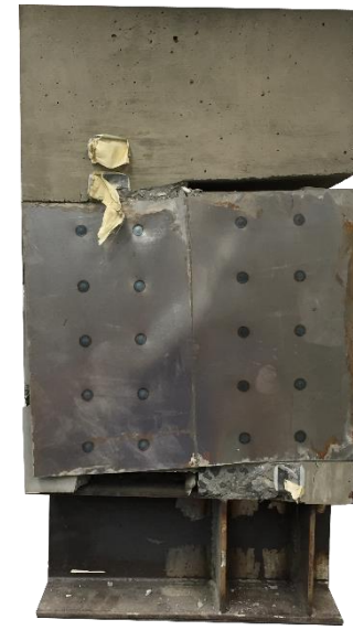
External Steel Plate \rho=0.75\% t=0.094 in. (13 gage)
