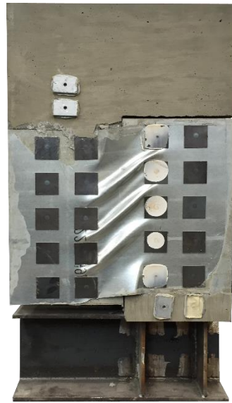
External Steel Plate \rho=0.25\% t=0.031 in. (22 gage)
