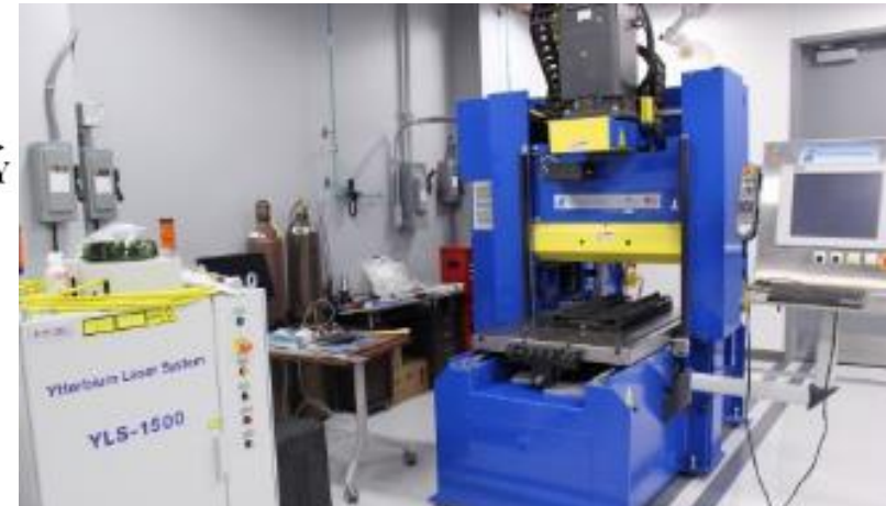
Friction Stir- Laser Hybrid Machine at CFSP
