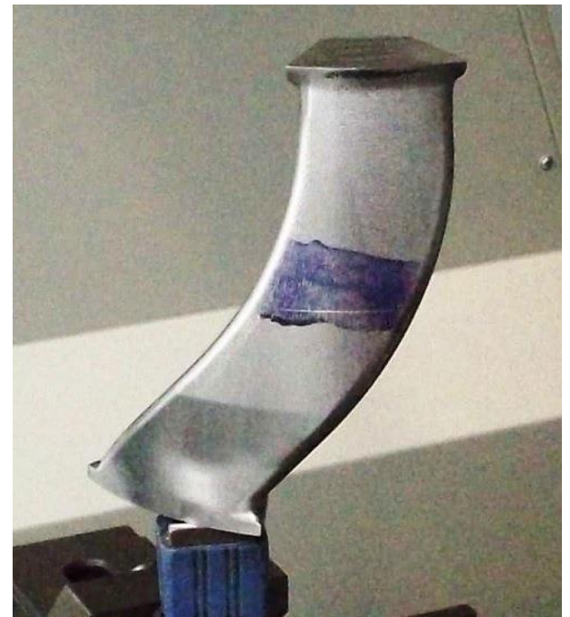
Vane Insert—one of 8 that fit into the swirler
