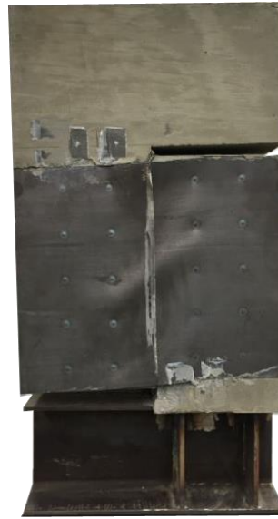
External Steel Plate \rho=0.50\% t=0.063 in. (16 gage)
