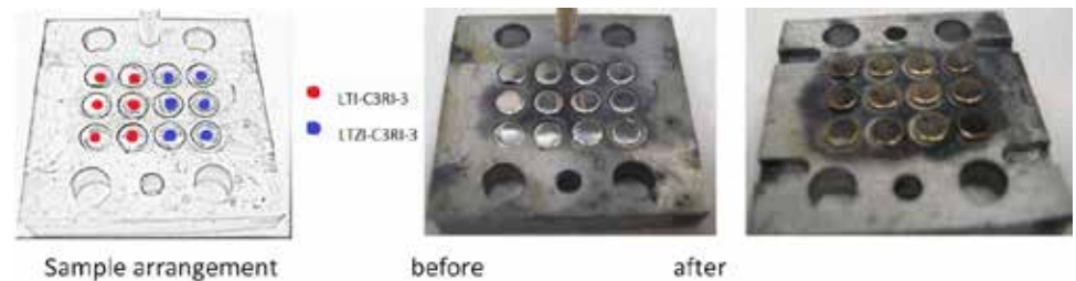
Fig. 2: Picture of L-alloys before and after proton implantation.
