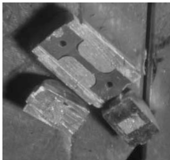
Sample retrieval at HFEF showing problems for Capsule-G, 100°C, 1 dpa
